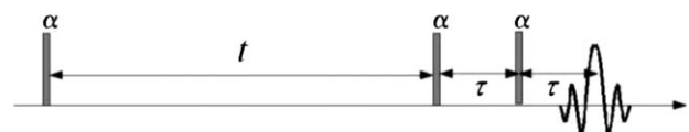
Fig. 5. Echo-detected saturation-recovery sequence used for slice-selective relaxation time measurement in a static magnetic field gradient. The pulse angle \alpha was determined from maximizing the signal intensity in a spin-echo experiment.
